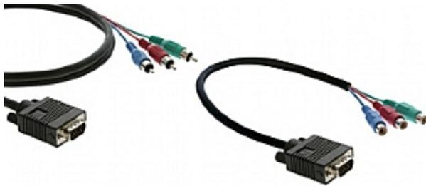
Kramer's computer graphics video to component video breakout cables are constructed from 3 mini coax cables with a 15-pin HD (M) connector at one end and 3 RCA (M or F) connectors at the other. These cables send or receive computer graphics video or component video signals.
