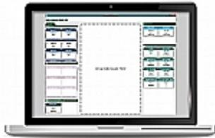
**EDID Designer** is a powerful and versatile software application for viewing, editing and uploading extended display identification data (EDID) to compatible Kramer devices. EDID is used in most of today's VGA, HDMI and DVI systems to maintain the video signal integrity between source and display. The application is mainly a setup tool designed for trained and experienced personnel who are familiar with EDID concepts to ensure signal integrity in their AV setups.
