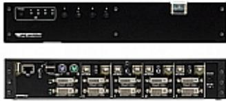
The **K244E** is a secure 4-port, DVI-I dual-display KVM switch. It provides the highest possible isolation between four connected computers each having two video output ports. The video ports support various video interfaces, from VGA to dual-link DVI and HDMI. Each computer may connect to up to two independent displays and operate in dual-display mode.
