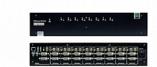
The **K248E** is a secure 8-port, DVI-I dual-display KVM switch. It provides the highest possible isolation between eight connected computers each having two video output ports. The video ports support various video interfaces, from VGA to dual-link DVI and HDMI. Each computer may connect to up to two independent displays and operate in dual-display mode.
