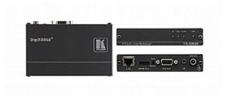
TP-580R is a high-performance, long-reach HDBaseT receiver for 4K60Hz (4:2:0) HDMI, RS-232 and IR signals over twisted pair. It extends video signals to up to 40m (130ft) over CAT copper cables at up to 4K@60Hz (4:2:0) 24bpp video resolution and provides even further reach for lower HD video resolutions.
