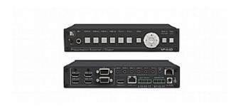
The VP-440 is a high-performance presentation scaler/switcher with four HDMI and two computer graphics (VGA) inputs. The unit scales the video, embeds the audio and outputs the signal to an HDMI output and an HDBaseT output simultaneously. The unit includes analog and embedded audio inputs and outputs.
