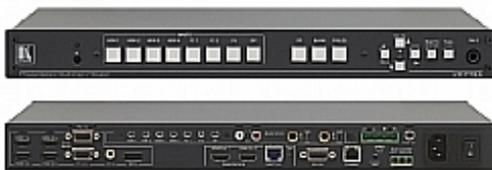
The VP-773A is a high-performance presentation switcher and scaler. It accepts one of eight inputs: one DisplayPort (DP), one composite video, two computer graphics and four HDMI signals. It scales the video, embeds the audio, and simultaneously outputs the signal to two identical HDMI and one HDBaseT TP output, together with S/PDIF and balanced stereo audio outputs. The unit also includes an audio amplifier and speaker outputs.
