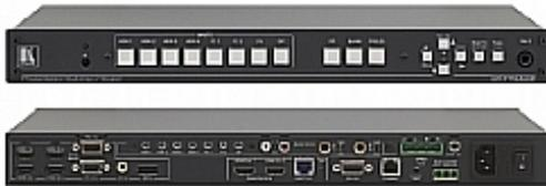
The **VP-773AMP** is a high-performance presentation switcher and scaler. It accepts one of eight inputs: one DisplayPort (DP), one composite video, two computer graphics and four HDMI signals. It scales the video, embeds the audio, and simultaneously outputs the signal to two identical HDMI and one HDBaseT TP output, together with S/PDIF and balanced stereo audio outputs. The unit also includes an audio amplifier and speaker outputs.
